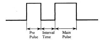
Figure 2. Double Pulse Wave Form
