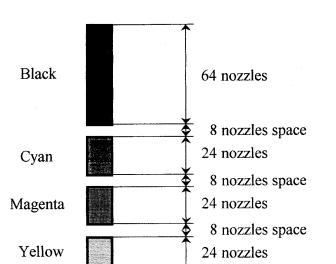
Figure 4. BC21 (Color Head for BJC-4000) Nozzle Layout
