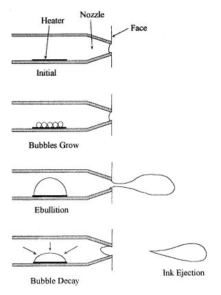
Figure 1. Ink Ejection of Bubble-jet printer
